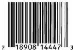
There are several bar code formats used for different purposes. The retail trade generally uses the -A format to mark consumer goods. Laser discs and DVDs are marked with this variety, which consists of a 12 digit number. The contents of the UPC-A code may be understood as follows:
